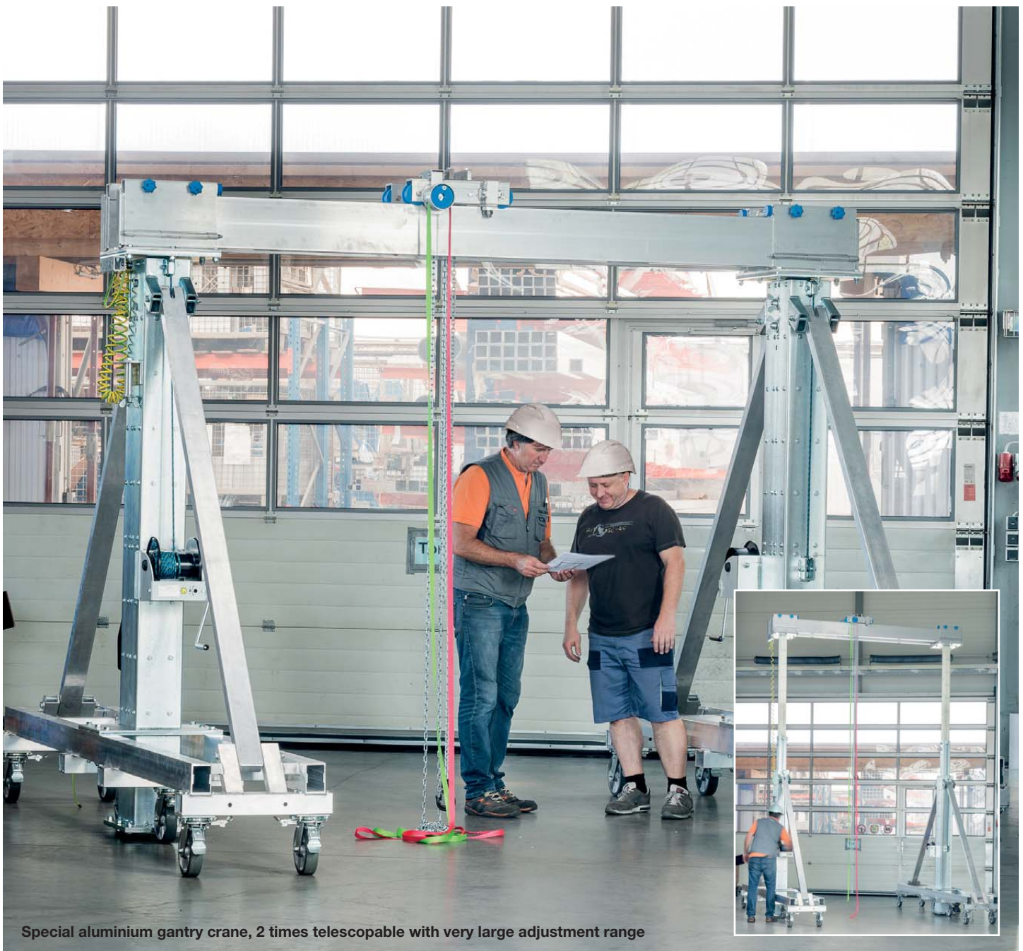
Special aluminium gantry crane, 2 times telescopic with very large adjustment range
