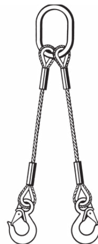
2-leg wire rope sling with master links and safety hook
