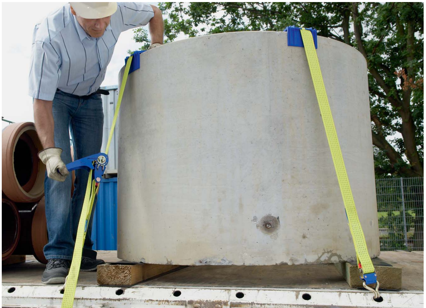
Structure of endless lashing strap
