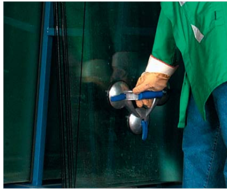
Suction lifters for handling of glass plates etc.
