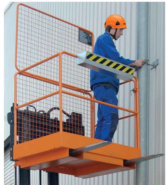
SIKO: Crosswise pick-up by forklift truck
