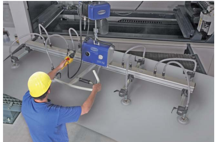
VacuMaster Basic for horizontal handling, 250 kg load
